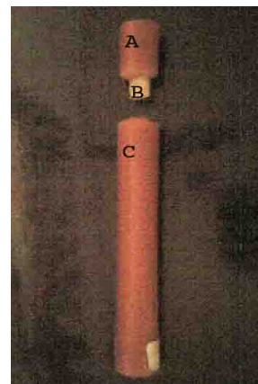
Figure 7. Sample after testing. A. Jig; B. Acrylic artificial teeth; C. Prosthetic base simulation.
