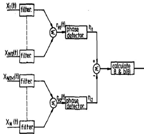
Fig 7. Split Beam Processor to obtain estimates of the incidence angle and the beam pattern factor, Source in (Ehrenberg, 1979)
