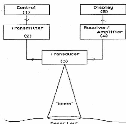
Fig 1. Working mode of hydroacoustic tool
