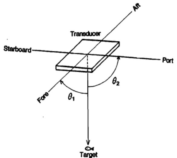
Fig 4. Geometry targets in Split Beam transducer. Towards the target defined by the  $\theta_1$  and  $\theta_2$  angle, Source in (MacLennan and Simmonds, 1992).
