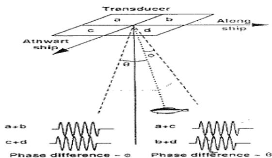
Fig 3 Split beam shape and a full beam transducer, Source in (MacLennan and Simmonds, 1992)
