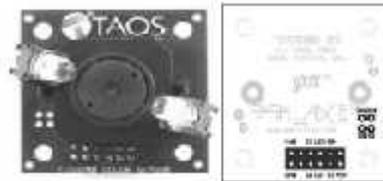
Gambar 1. Sensor warna TCS3200-DB
