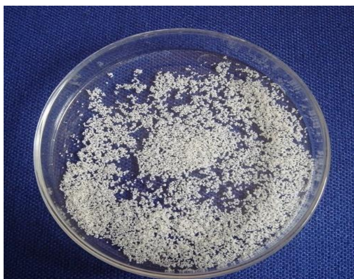
Figure 3: Prepared hollow microspheres of DBM.
