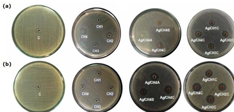
Figure 5. Inhibitory zone of chitosan (C), chitosan hydrolysate (CH) and silver nanoparticles (Ag/CH) toward (a) S. Aureus and (b) E. coli
