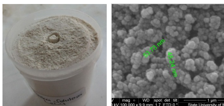
Figure 1. The appearance of silica-cellulose material (left) and the SEM picture of the same material at 80.000 times magnification
