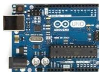
Gambar 3. Arduino Uno R3 Board
