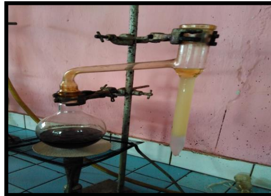
Gambar 8. Hasil Proses Destilasi Kadar Air Aspal Buton
