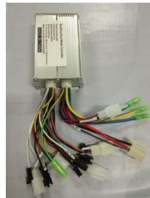
Gambar 3. Controller BLDC 350W
