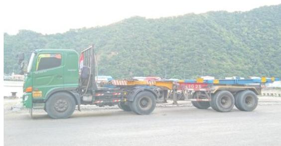
**Gambar 5.** Alat angkut *head truck* (Sumber: PT. Pelindo, 2022)
