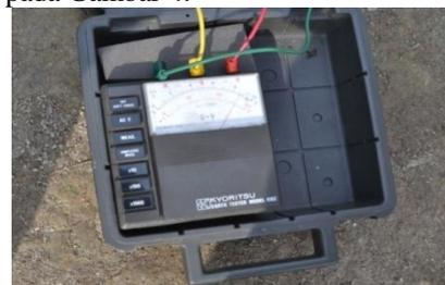
Gambar 2. Alat ukur Earth Tester model 4182 merek Kyoritsu
