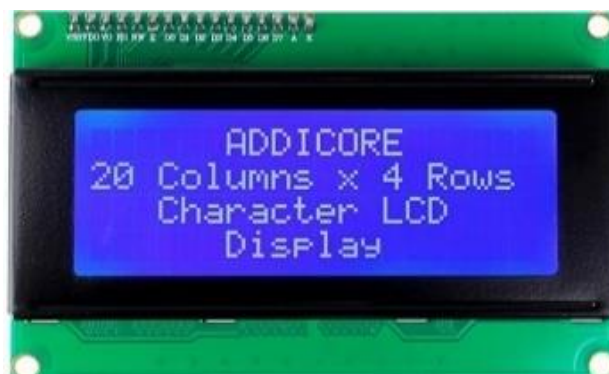
Fig. 5 Illustration of LCD 20x4.
