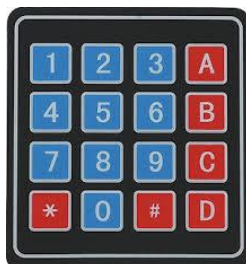
Fig. 2 Illustration of Module of Keypad 4x4.
