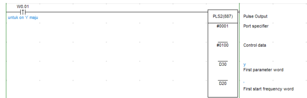
Figure 7. Ladder diagram of running a stepper motor
