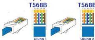
**Gambar 5. Kabel *Straight* Tipe T568**
