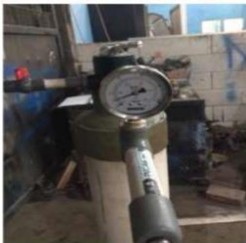
Gambar 4.2. Proses Hidrotest Tabung PreTreatment Filter RO 400 GPD
