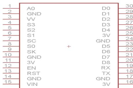
NodeMCU is basically an extension of the ESP 8266 with e-Lua based firmware. The NodeMcu is equipped with a micro usb port that functions for programming and power supply. In addition, the NodeMCU is equipped with a push button, namely the reset and flash buttons. NodeMCU uses the Lua programming language which is a package of esp8266. The Lua language has the same logic and programming structure as C, only the syntax is different. If you use Lua then you can use.
