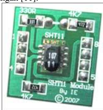
Gambar 2. Modul DT sense SHT11 Sumber [12]
