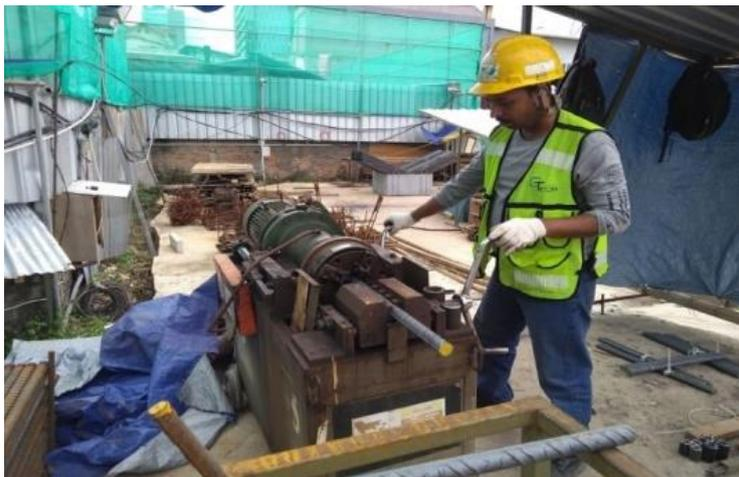
Gambar 9. Proses Threading Ulir
