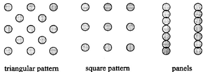
**Gambar 4** Pola *deep soil mix* (DSM)
