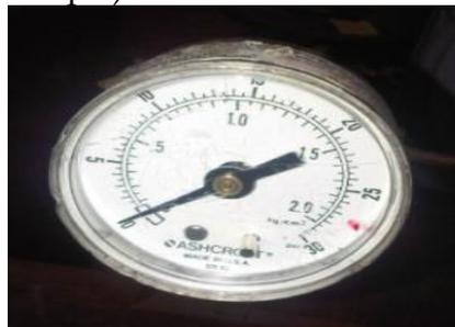
Gambar 3. *Pressure gauge Suction*
