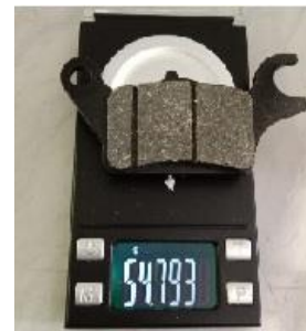
Figure 11. Weighing brake pads
