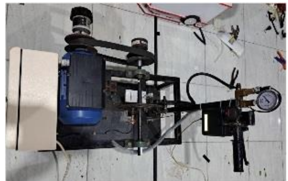
Figure 8. Brake Lining Thickness Experimental Test Tool
