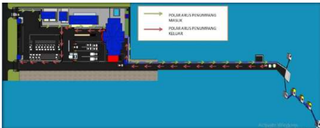
Figure 3 Planned Passenger Traffic Flow Patterns Description of the drawing up and down of passengers:
