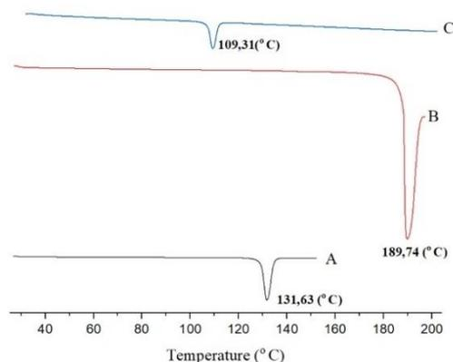
**Figure 1.** Thermogram overlay of piperine (A), succinic acid (B), and piperine-succinic acid cocrystal (C)
