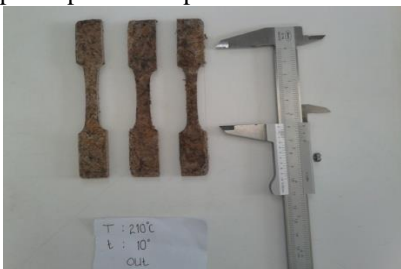
Gambar 4. Sampel uji tarik
