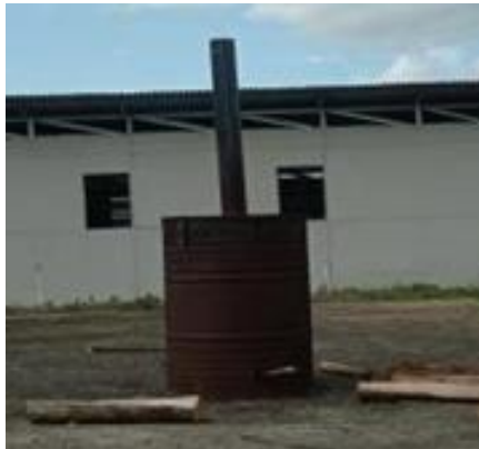
Gambar 3. Drum kiln tertutup/pirolisis
