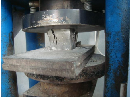
Gambar 1 Pengujian Kuat Tekan Mortar B. Pemodelan Artificial Neural Network (ANN)
