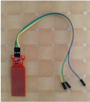
Gambar 6. Water Level Sensor
