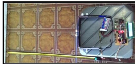
**Gambar 13.** Proses pengujian sensor ultrasonik SRF04
