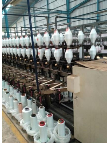
Figure 4.6 Thread passing process on Mc.PW
