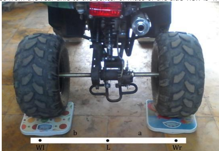
Figure 2 Weighing the front and rear axle rear view
