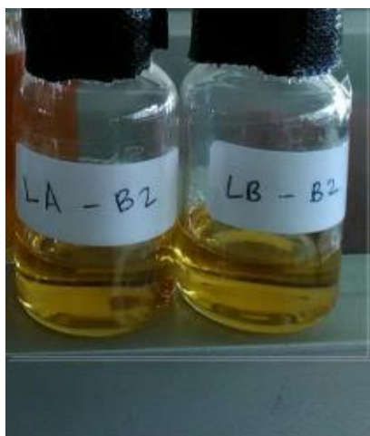
Figure 4. Obtained biodiesel from castor oil transesterification catalyzed by lithium intercalated bovine bone catalyst (Li- 3 wt%)
