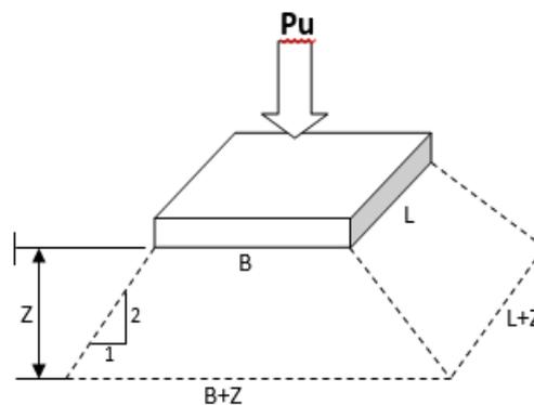
Figure 2. Illustration of stress distribution due to loading with 2V:1H distribution method (2 vertical units versus 1 horizontal unit)
