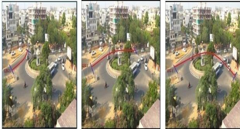
Figure 3 Possible movements at a roundabout (Sonu et al. , 2016)
