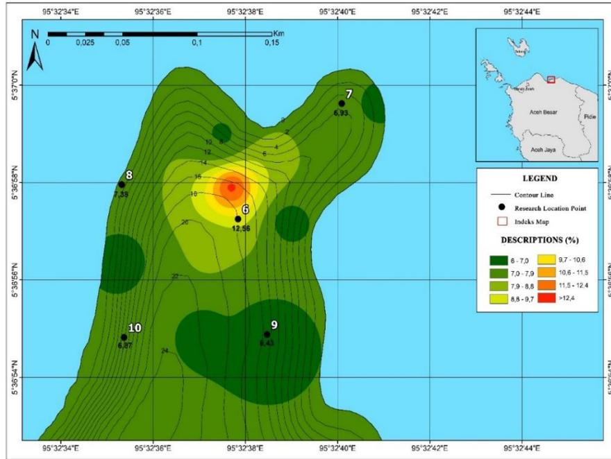
Figure 8. GIS Analysis of  $\text{CaCO}_3$  contours at station 2 of Lamreh Cliff
