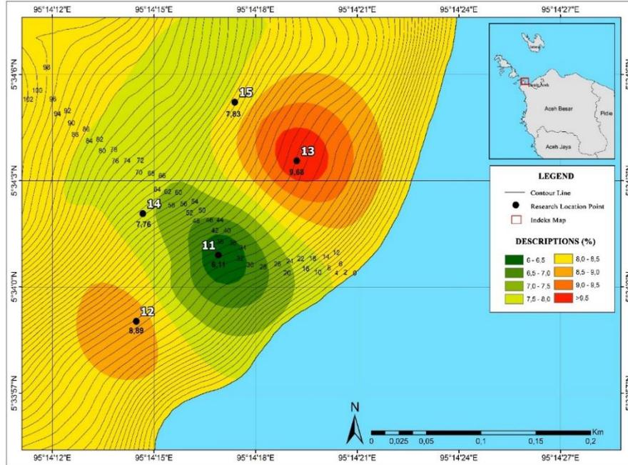
Figure 9. GIS Analysis of  $\text{CaCO}_3$  contours at station 3 of Ujong Pancu Cliff.
