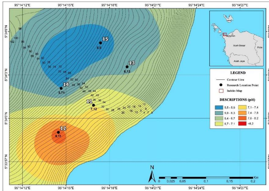
**Figure 13.** GIS Analysis of soil pH contours at station 3 of Ujong Pancu Cliff.
