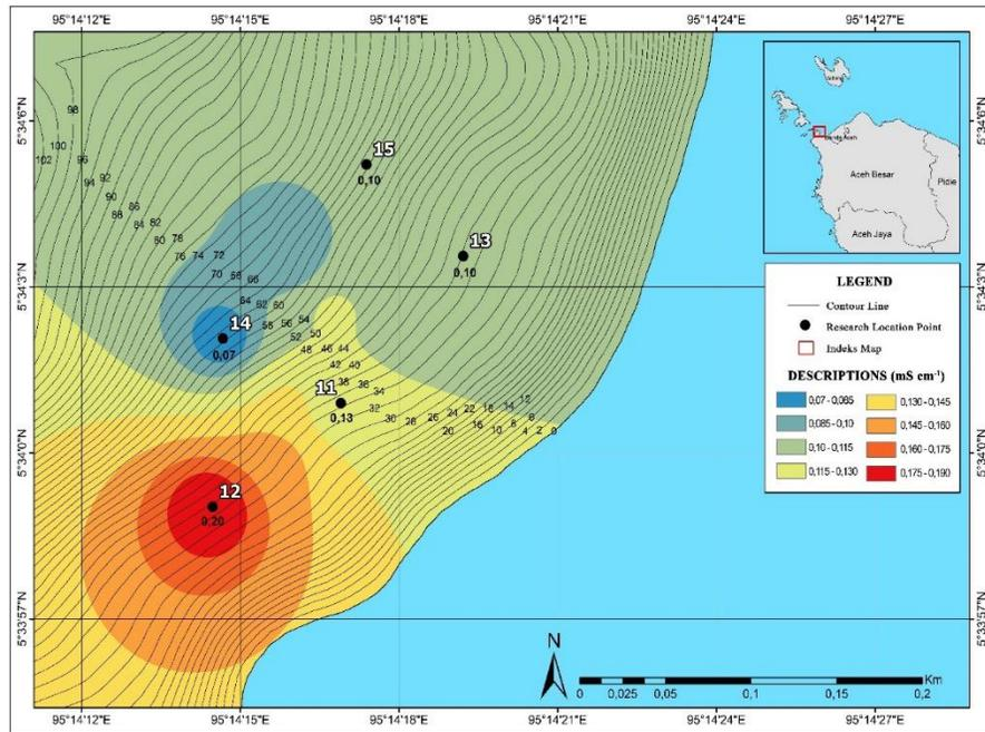
**Figure 17.** GIS Analysis of soil salinity contours at station 3 of Ujong Pancu Cliff.
