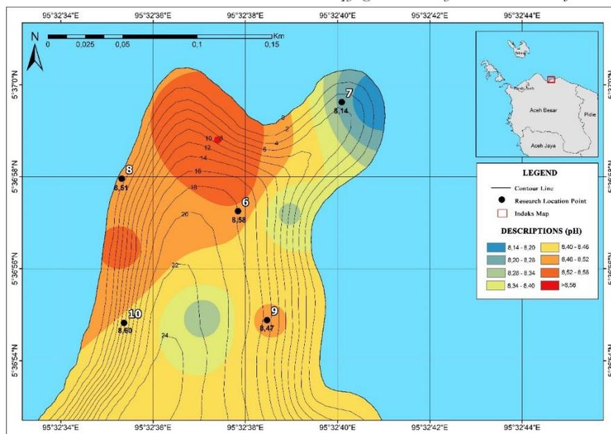
Figure 12. GIS Analysis of soil pH contours at station 2 of Lamreh Cliff.
