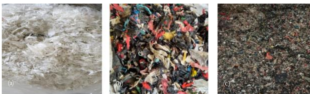
Figure 3. Typical shreds and quality of LDPE plastic used: (a) white LDPE; (b) mix-plastic LDPE; (c) Blend-plastic LDPE.
