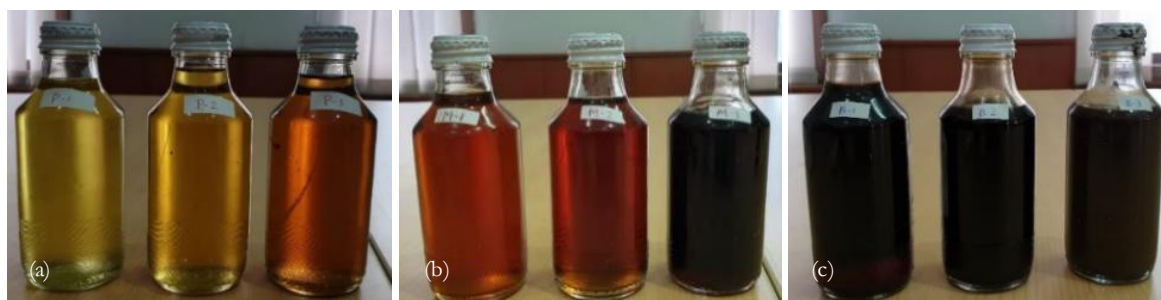
Figure 4. Visualization of oil produced from LDPE plastic pyrolysis: (a) LDPE Plastic Oil: MP-1, MP-2, and MP-3; (b) Mix Oil of LDPE Plastic: MM-1, MM-2, and MM-3; (c) Blend Oil of LDPE Plastic: MB-1, MB-2, and MB-3.
