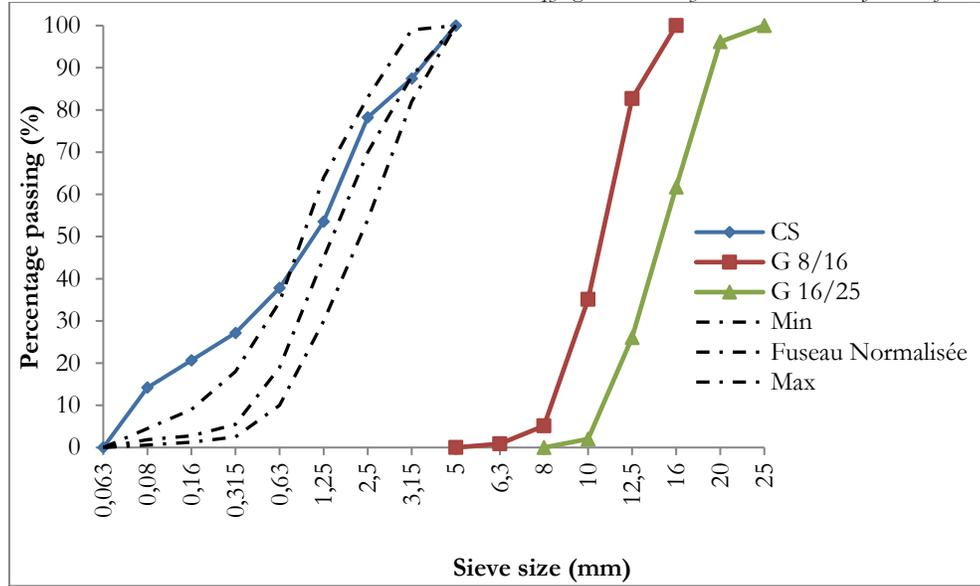
**Figure 1.** Grading curves of gravel and crushed sand compared with the normalized curve
