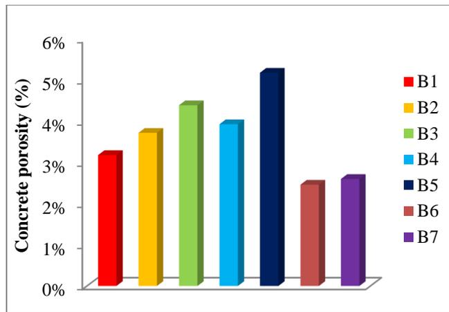
**Figure 4.** Concrete porosity of mixtures without and with expanded clay aggregates. B1 (100% S+100%G1+100%G2); B2 (100%S+ 85%G1+15% ECA 1+ 100%G2); B3 (100%S+ 70%G1+30% ECA 1+100%G2 ); B4 (100%S+ 100%G1 + 85%G2+15% ECA 2 ); B5 (100%S+ 100%G1 +70%G2+30% ECA 2 ); B6 (85%S+ 15% ECA 3 + 100%G1 + 100%G2); B7 (70%S+ 30% ECA 3 + 100%G1 + 100%G2)
