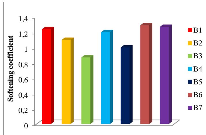
**Figure 5.** Softening coefficient of mixtures without and with expanded clay aggregates. B1 (100% S+100%G1+100%G2); B2 (100%S+ 85%G1+15% ECA 1+ 100%G2); B3 (100%S+ 70%G1+30% ECA 1+100%G2 ); B4 (100%S+ 100%G1 + 85%G2+15% ECA 2 ); B5 (100%S+ 100%G1 +70%G2+30% ECA 2 ); B6 (85%S+ 15% ECA 3 + 100%G1 + 100%G2 ); B7 (70%S+ 30% ECA 3 + 100%G1 + 100%G2)
