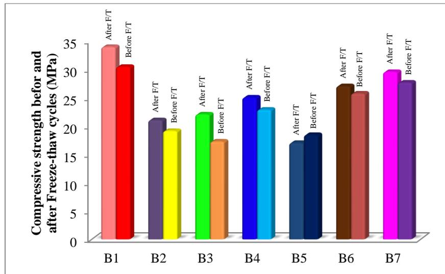
**Figure 7.** Compressive strength of concrete mixtures without and with ECA before and after freeze-thaw cycles. B1 (100% S+100%G1+100%G2); B2 (100%S+ 85%G1+15% ECA 1+100%G2); B3 (100%S+ 70%G1+30% ECA 1+100%G2 ); B4 (100%S+ 100%G1 + 85%G2+15% ECA 2 ); B5 (100%S+ 100%G1 +70%G2+30% ECA 2 ); B6 (85%S+ 15% ECA 3 + 100%G1 + 100%G2 ); B7 (70%S+ 30% ECA 3 + 100%G1 + 100%G2)
