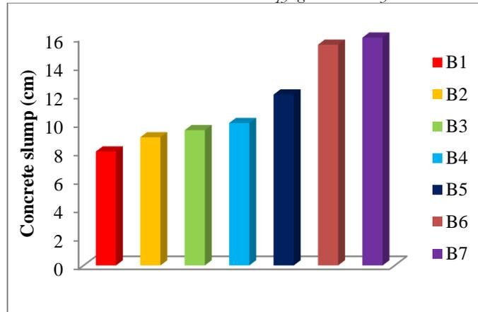
**Figure 3.** Slump test results of concrete without and with expanded clay aggregates. B1 (100% S+100%G1+100%G2); B2 (100%S+ 85%G1+15% ECA 1+ 100%G2); B3 (100%S+ 70%G1+30% ECA 1+100%G2 ); B4 (100%S+ 100%G1 + 85%G2+15% ECA 2 ); B5 (100%S+ 100%G1 +70%G2+30% ECA 2 ); B6 (85%S+ 15% ECA 3 + 100%G1 + 100%G2); B7 (70%S+ 30% ECA 3 + 100%G1 + 100%G2)
