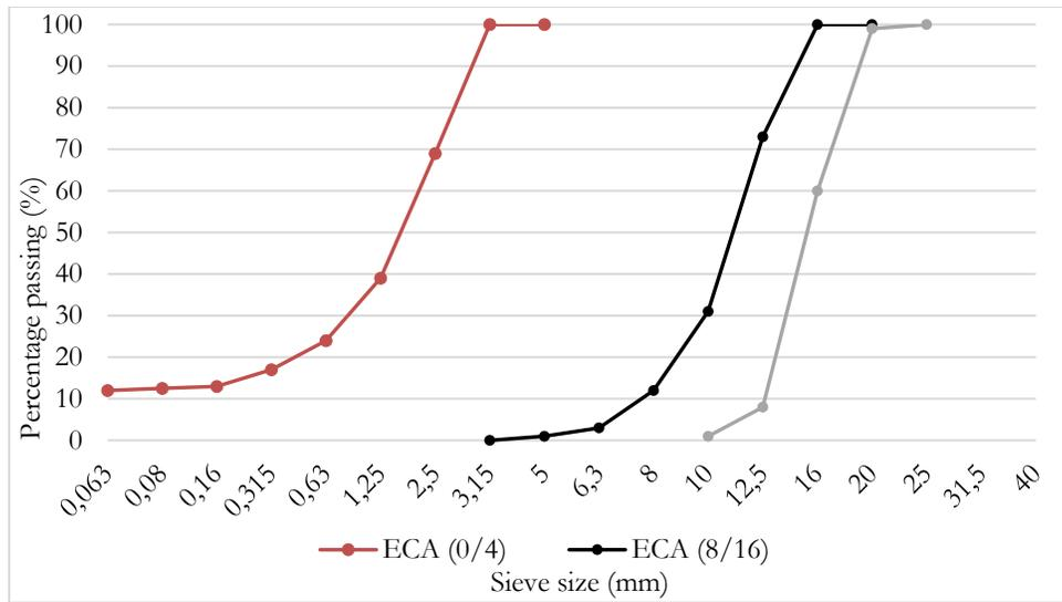
**Figure 2.** Grading curves of Expanded clay aggregates (0/4 mm, 8/16 mm, and 16/25 mm)
