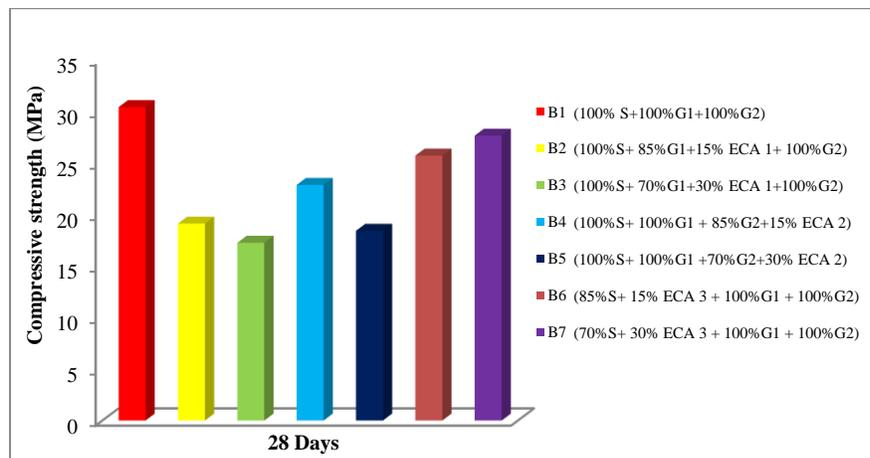
**Figure 6.** Compressive strength of concretes without and with expanded clay aggregates. B1 (100% S+100%G1+100%G2); B2 (100%S+ 85%G1+15% ECA 1+ 100%G2); B3 (100%S+ 70%G1+30% ECA 1+100%G2 ); B4 (100%S+ 100%G1 + 85%G2+15% ECA 2 ); B5 (100%S+ 100%G1 +70%G2+30% ECA 2 ); B6 (85%S+ 15% ECA 3 + 100%G1 + 100%G2 ); B7 (70%S+ 30% ECA 3 + 100%G1 + 100%G2)
