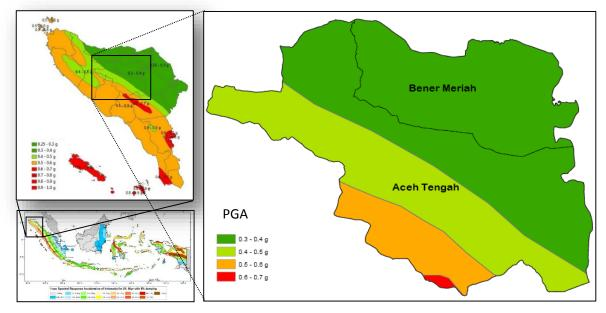
**Figure 1.** Peak Ground Acceleration in bedrock for Aceh Tengah and Bener Meriah Seismic Hazard Map with Spectral period = 1 second for 2% probability of exceedance (PE) in 50 years in bedrock (Tim Revisi Peta Gempa Indonesia, 2010).
