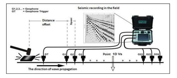
Figure 2. Process of MASW Seismic measurements using seismometers 24 geophones (Rusydy, Khaizal, Fatimah, Syafrizal, & Andika, 2016)
