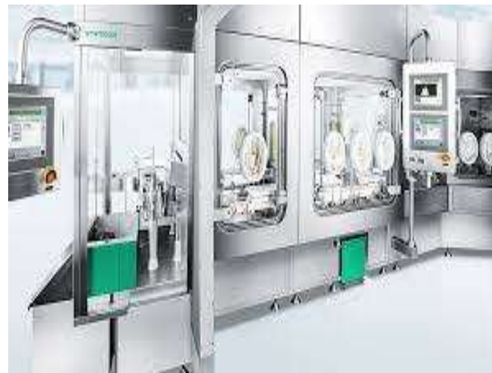
Figure 2. ALF 5080 barrier technology
