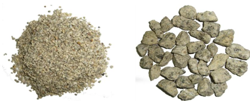
Figure 2. Recycled Concrete Aggregate (a) Fine RCA (b) Coarse RCA.
