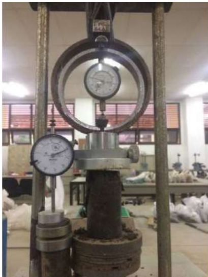
Figure 1 Unconfined Compressive Strength Test at Unsyiah Soil Mechanics Laboratory
