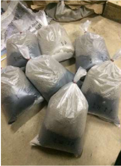
Figure 2 Sample of Soil that Has Been Mixed with Pumice Powder and Wood Charcoal Powder
