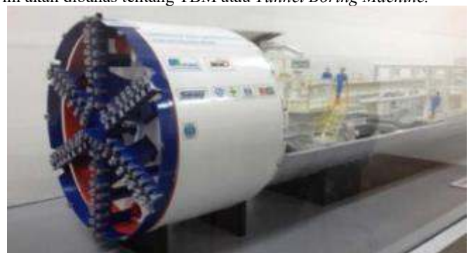
Gambar 20. Tunnel Boring Machine
