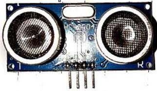
Gambar 5. Sensor ultrasonik
