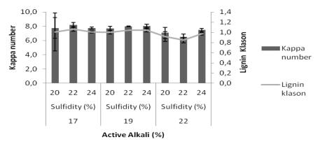
Figure 2 The effect of active alkali and sulfidity loading on Kappa number and klason lignin of pulp
