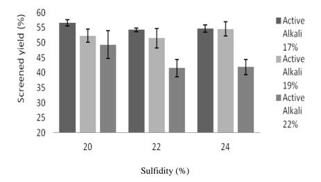
Figure 1 The efect of active alkali and sulfidity loading on screened pulp yield
