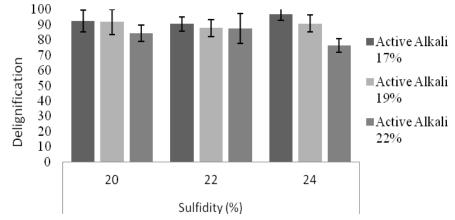
Figure 4 The efect of active alkali and sulfidity laoding on delignification selectivity of pulp
