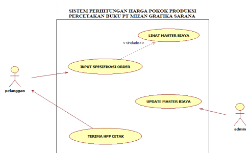
Gambar. 1 Use case sistem perhitungan HPP
