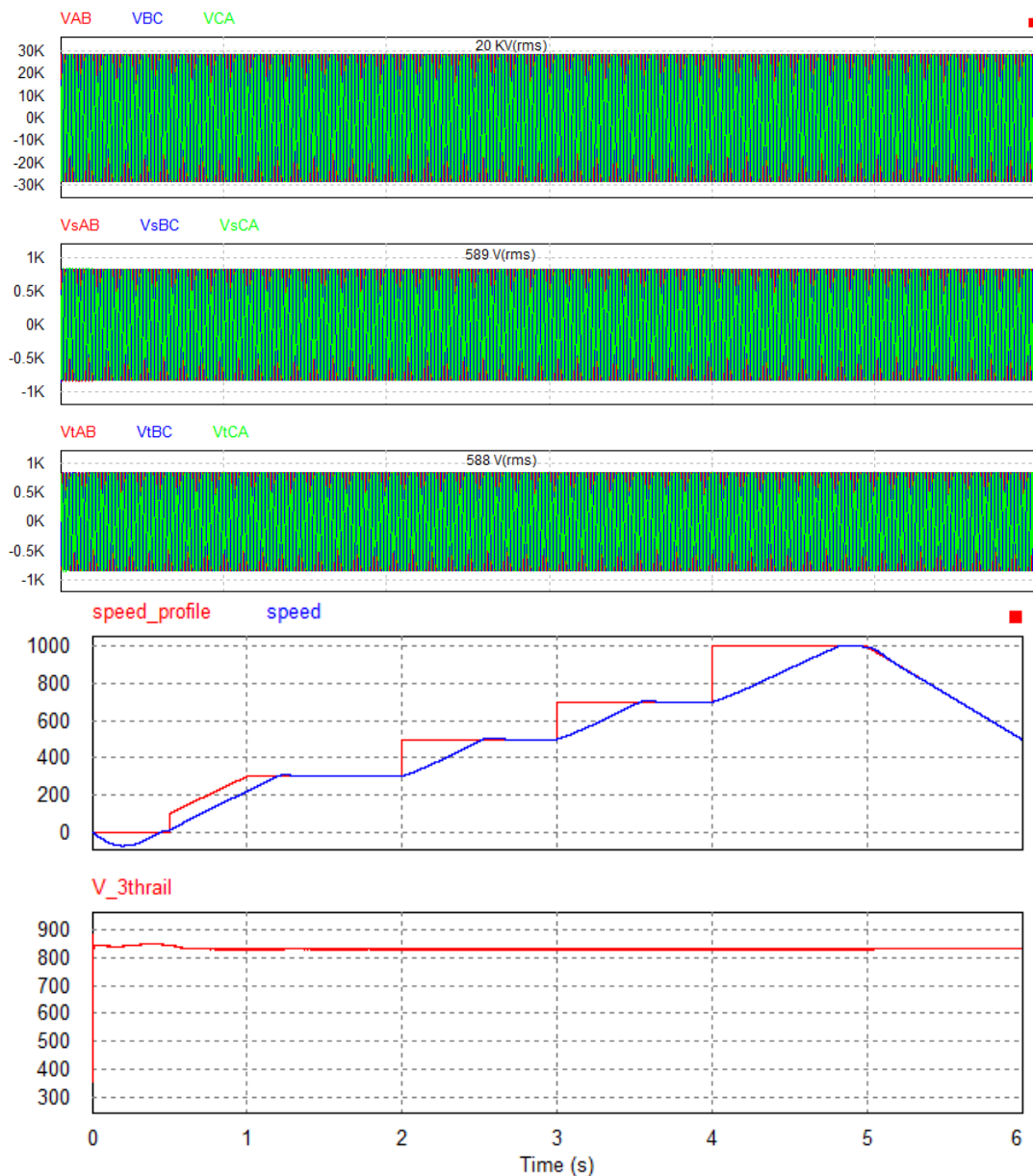
Figure 5. Voltage Profile Measurement when 3 phase induction motor with VFD has been connected with varous speed operation
