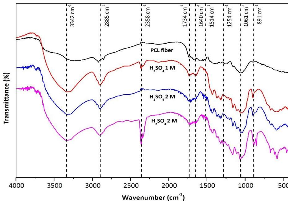
**Figure 1.** FTIR spectra of microcrystalline cellulose from pineapple crown leaf waste hydrolyzed with 1, 2, and 3 M concentrations of sulfuric acid.
