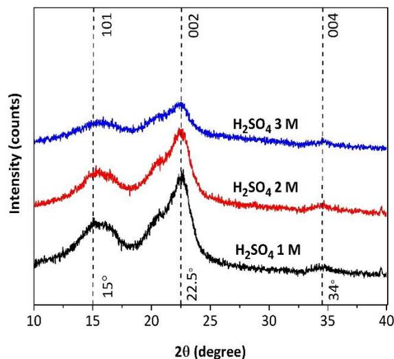
**Figure 3.** X-ray diffraction patterns of microcrystalline cellulose from pineapple crown leaf waste hydrolyzed with 1, 2 and 3 M concentrations of sulfuric acid.
