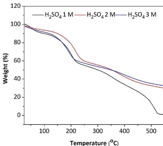
**Figure 4.** Thermogram of microcrystalline cellulose from pineapple crown leaf waste hydrolyzed with 1, 2 and 3 M concentrations of sulfuric acid.
