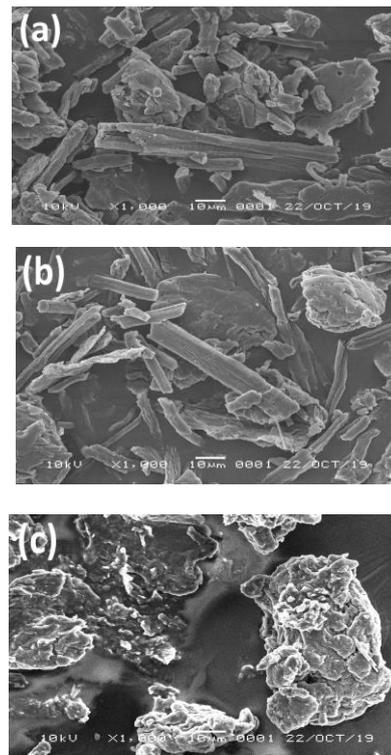
**Figure 2.** Micrographs of microcrystalline cellulose from pineapple crown leaf waste with (a) 1 M, (b) 2 M, and (c) 3 M acid concentrations.
