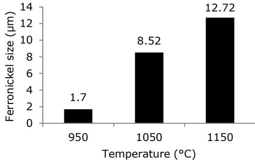
**Figure 10.** The effect of reduction temperature in particle size of feronickel
