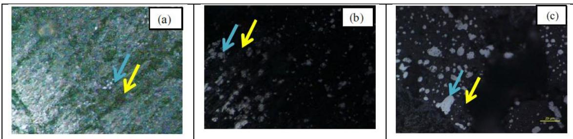
**Figure 9.** Microstructure of reduced nickel ore with 10 wt. % Na<sub>2</sub>SO<sub>4</sub> additive and 10 wt. % reductant for 60 minute in various reduction temperatures: (a) 950°C, (b) 1050°C dan (c) 1150°C
