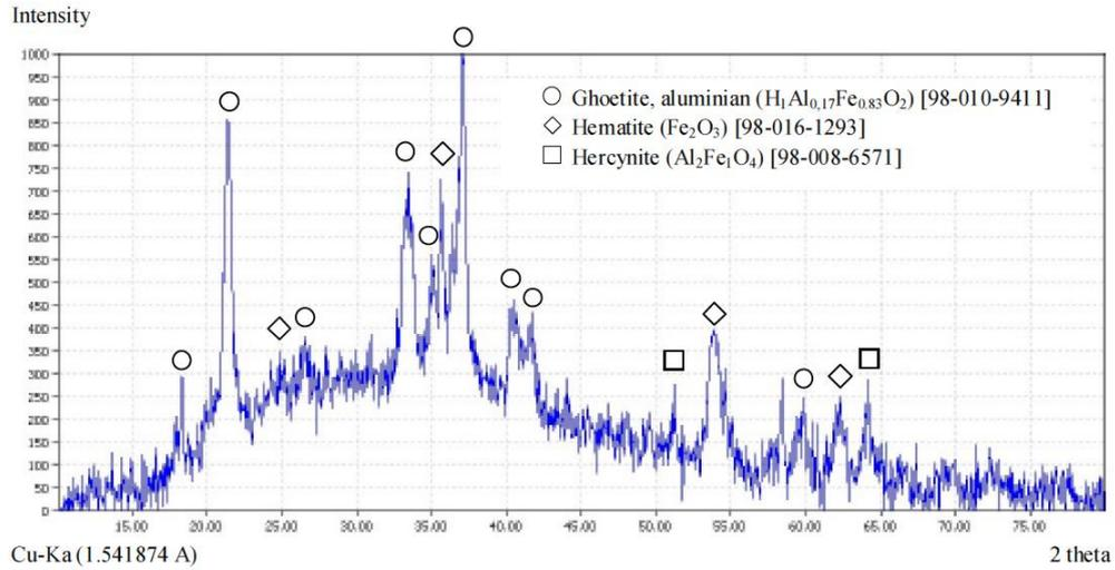
Figure 2. XRD analysis of low-grade lateritic nickel ore
