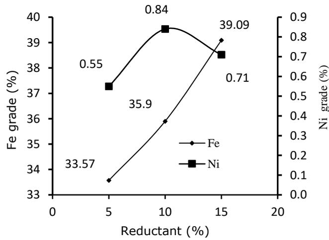
Figure 3. Effect of the number of reductant on iron and nickel grade with 10 wt. % additives of sodium sulfate at reduction temperature of 1050°C for 120 minutes
