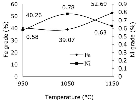
**Figure 7.** Effect of temperature on iron and nickel grade with 10 wt. % additives of  $\text{Na}_2\text{SO}_4$  at reduction 60 minutes and reducing agents 10 wt. %
