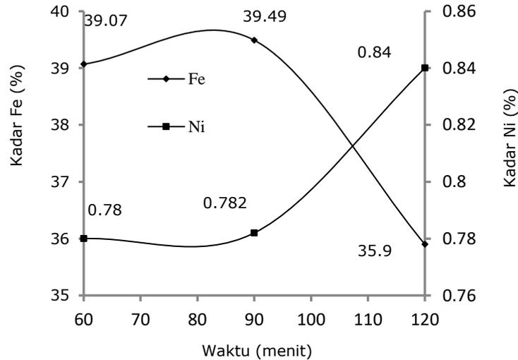
**Figure 11.** Effect of reduction time on selective reduction low-grade nickel ore with 10 wt. % additives of sodium sulfate and 10 wt. % of reductant at reduction temperature of 1050°C.
