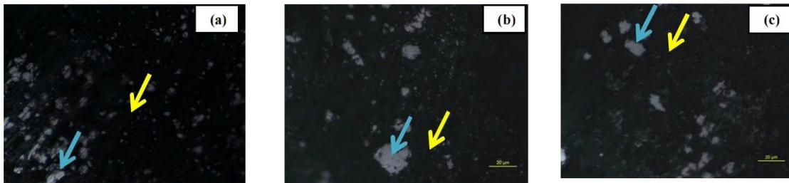
**Figure 13.** Microstructure analysis of reduced nickel ore with the addition of 10 wt. % sodium sulfate and 10 wt. % of reductant at reduction temperature 1050°C for: (a) 60 minutes, (b) 90 minutes dan (c) 120 minutes
