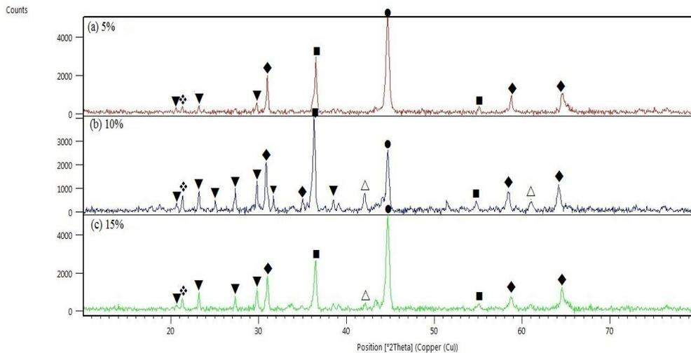
Figure 4. The XRD patterns of reduced pellets at 1050°C for 120 minutes with 10 wt.% additives of sodium sulfate with various number of reductant: (a) 5 wt.%, (b) 10 wt.% and (c) 15 wt.%. (▼=  $NaAlSiO_4$ , ■= $Al_2FeO_4$ , ●= $FeNi$ , ◆= $Fe_2MgO_4$ , △= $FeO$ , ❖= $SiO_2$ )
