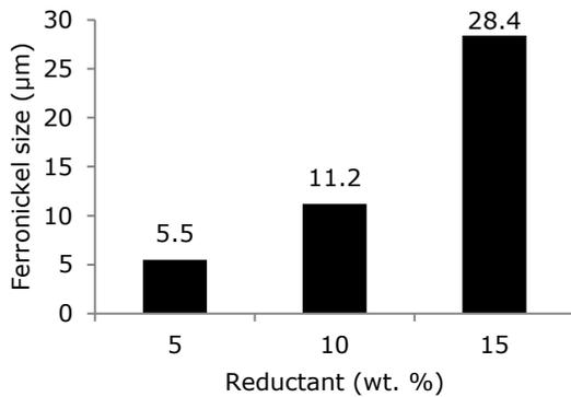
**Figure 6.** The effect of reductant amount in particle size of ferronickel.
