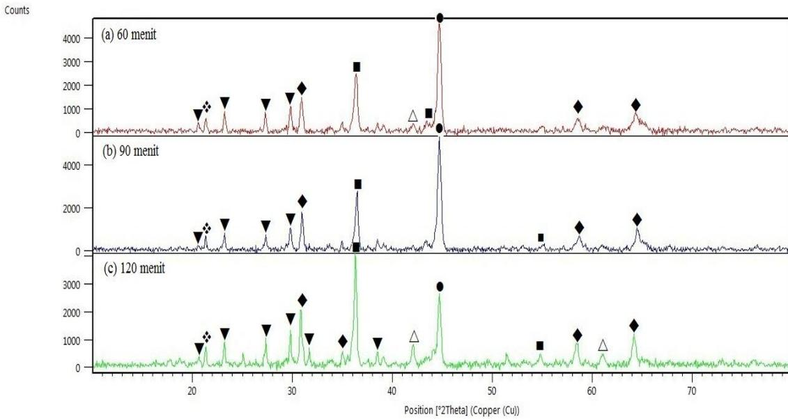
**Figure 12.** The XRD pattern of reduced nickel ore with the addition of 10 wt. % sodium sulfate and 10 wt. % of reductant at reduction temperature 1050°C for : (a) 60 menit, (b) 90 menit dan (c) 120 menit. (▼= NaAlSiO<sub>4</sub>, ■=Al<sub>2</sub>FeO<sub>4</sub>, ●=FeNi, ◆= Fe<sub>2</sub>MgO<sub>4</sub>, △= FeO, ◆= SiO<sub>2</sub>).
