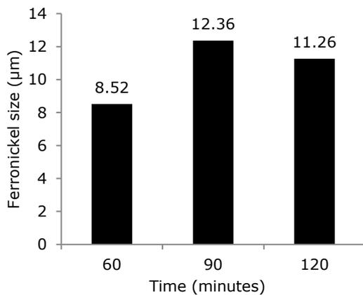
**Figure 14.** The effect of holding temperature in reduction process on the particle size of feronickel.
