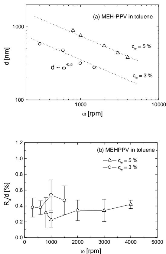
Fig.3 Dependence of thickness (a) and surface roughness (b) of MEH-PPV films on the spinning speed.
