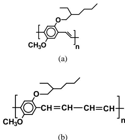
Figure 1. Molecular structure of MEH-PPV and MEH-PPB
