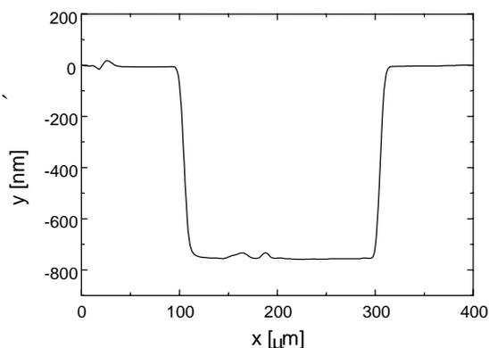
Fig. 2. Surface profile trace of MEH-PPV film of thickness of  $(749 \pm 10)$  nm prepared from toluene solution
