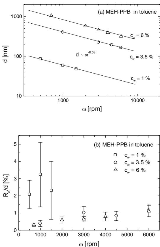
Fig. 4 Dependence of thickness (a) and surface roughness (b) of MEH-PPB films on the spinning speed.
