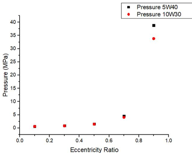
Fig. 8. Comparison chart of the ratio of eccentricity with maximum pressure.
