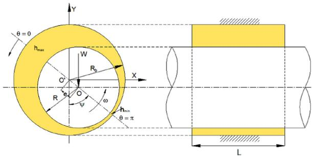
Fig. 1. Basic geometry of journal bearings [27].
