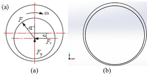
Fig. 3. Scheme load carrying capacity of oil film (a) model attitude angle equal to zero (b) modeling journal bearings.
