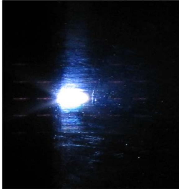
**Figure 1(c)** Cu plasma generated under surrounding air pressure of 760 Torr. The laser energy of 1,064 nm Nd-YAG laser was fixed at 100 mJ. The diameter of the plasma was around 4 mm.
